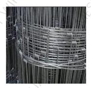
**Hinge joint fence** is a kind of fence, whose top and bottom wires are made of 2.5mm diameter wire, and the tensile strength is greater than or equal to 710N/mm2. The other wires are made of 1.9mm diameter wire, and the tensile strength is 440-540N/mm2.
