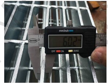
Bearing bar size inspection
